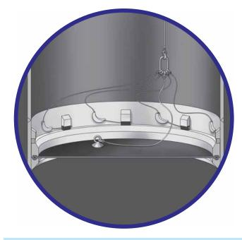
Diaphragms are fitted to top and bottom of sleeves to provide buoyancy of the sleeve during installation of the Jacket.
