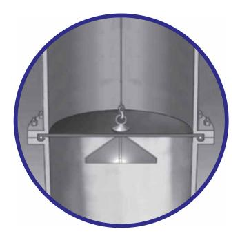
The function of Rip-Out Diaphragms is to accentuate the flooding of previously sealed jacket members or buoyancy tanks, by pulling a cruciform cutter through the diaphragm.
